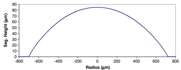
**Figure 5.** Surface profile for the photoresist microlens.
