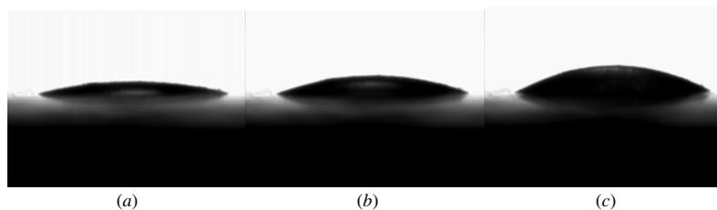
**Figure 8.** Photos for the curvature changes of the PDMS film lens with different volumes of pumped-in fluid: (a) initial position, (b) 20  $\mu\text{l}$  and (c) 45  $\mu\text{l}$ .
