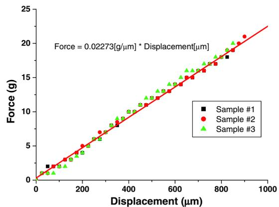
**Figure 6.** The plot for force versus displacement.
